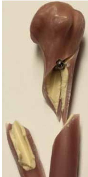
**Figure 3** A proximal humeral fracture involving the screw hole.
