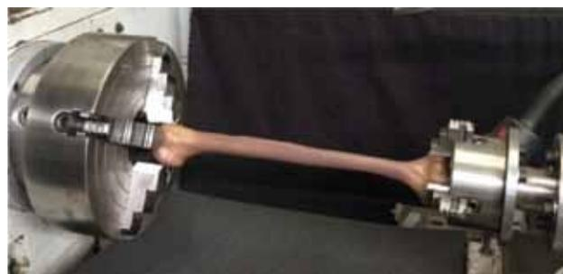
**Figure 2** A composite humerus is fixed in a modified lathe for assessing maximum and end torque.
