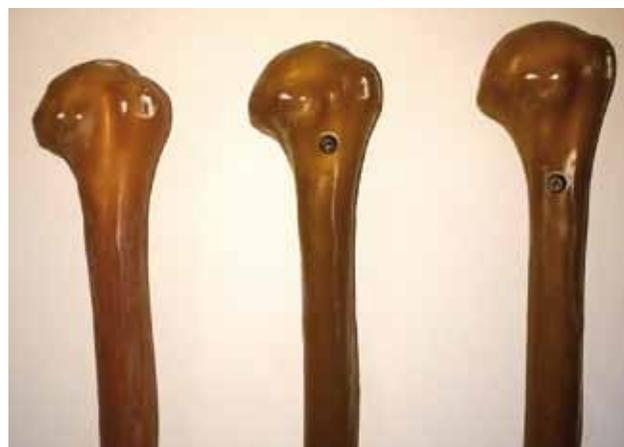
**Figure 1** Fourth-generation composite humerus model with no screw inserted or with a screw inserted in the distal (subpectoral) position or proximal (suprapectoral) position.
